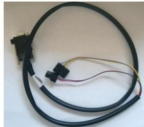
JCM's new RS 232C interface to connect JCM Products via USB Port.
