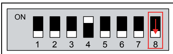
Figure 6-69 DIP SW1 #8 OFF
