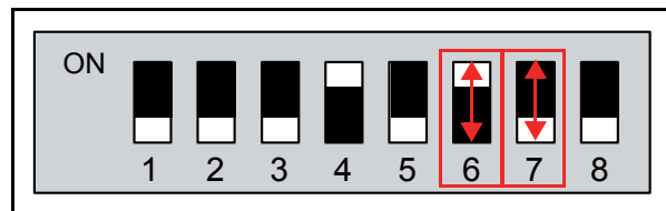
Figure 6-70 DIP SW1 #6 and #7 ON
